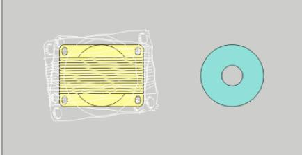
Toroidal transformers are also acoustically quieter than EI transformers. The absence of an air gap typically provides an 8:1 reduction of acoustic noise. In addition the windings tightly envelope the entire core, effectively reducing magnetostriction - the main source of the familiar mechanical hum found in standard vertically laminated EI transformers. Compared to EI transformers, toroids are silent.
