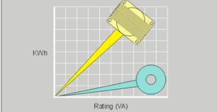
It takes a lot less energy to maintain the magnetic field in a toroidal core. This is known as excitation or quiescent power. Toroids require about 1/16 the excitation power of conventional transformers. That's 1/16 the electricity required by EI transformers in standby mode. This can translate into big savings in large transformer applications such as industrial controls.
