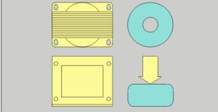
This efficiency yields the most easily identifiable feature of the toroid, its size benefit. Toroidal transformers are about half the size and weight of standard transformers.
